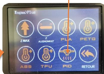
VOTRE IMPRIMANTE VA MONTER EN TEMPÉRATURE, CE QUI ALLUMERA VOTRE VENTILATEUR CENTRALE. UNE SÉRIE DE 8 PROTOCOLE VONT S'ENCLANCHER, IL VOUS SUFFIT D'ATTENDRE (10 À 15 MIN).
