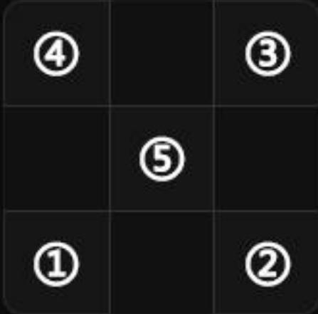
Press five buttons(① ... ⑤) to control nozzle moving to corners of bed.
