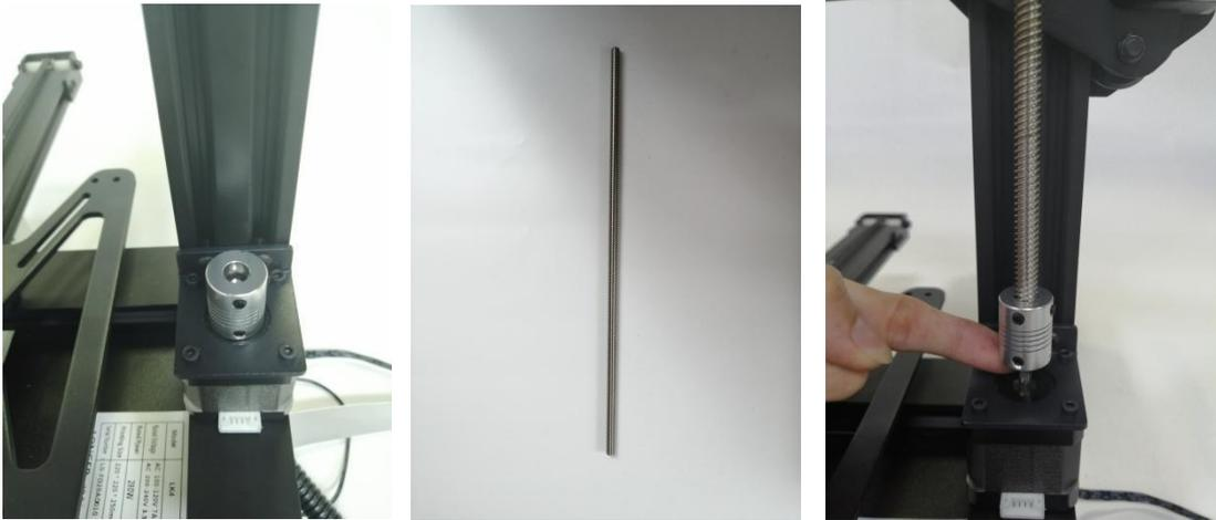
Let the lead screw snap into the coupling and the motor shaft is also aligned with the lead screw. Tighten the top wire
