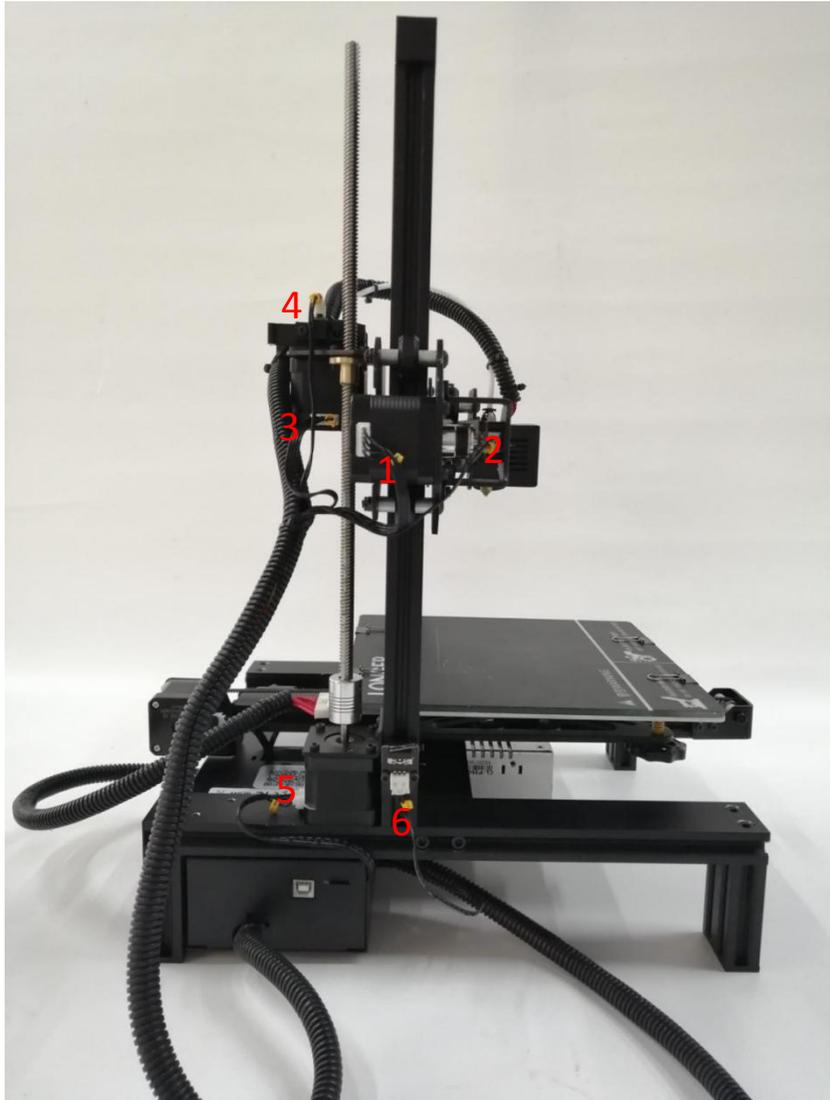
1. X motor line      2. X limit switch line      3. E-axis motor line
