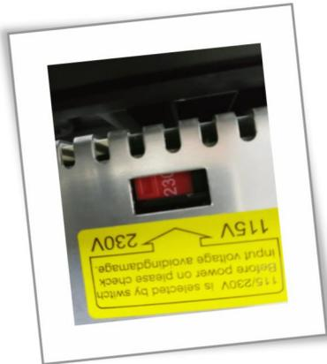
If the access voltage is 220V, please adjust the power supply in the control box to 220V, please be sure to confirm before powering on. Otherwise it will burn the power
