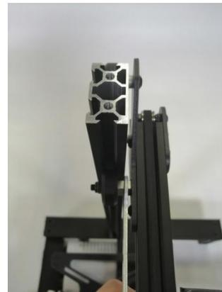
If the wheel does not fit in, you can adjust the wheel with the eccentric nuts on both sides. Let the X-axis beam enter
