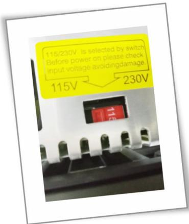
If the access voltage is 110V, please adjust the power supply in the control box to 110V, please be sure to confirm before powering on. Otherwise it will burn the power
