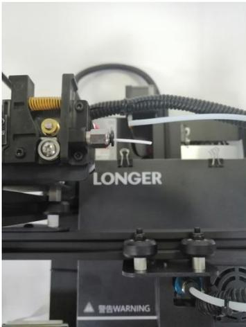
1. Before returning the material, please heat the nozzle first, and then withdraw the consumables as soon as possible. If you can't pump it, you can re-feed the material with the advanced material, and melt the extruded block formed at the end of the consumable in the nozzle.
