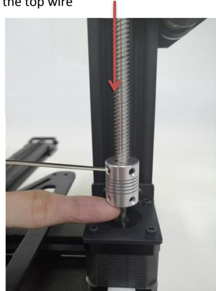
Adjust the screw movement by adjusting these two screws. The two screws cannot be tightened too tightly. Turn the coupling by hand to adjust the movement of the lead screw.
